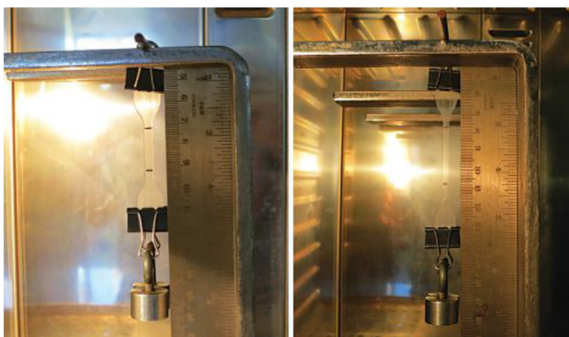
Fig. 10 — Specimen prepared for hot set test.
